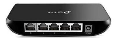
Step 3: Plug in one end of each of the provided ethernet cables into any of the open ports on the ethernet Switch.
